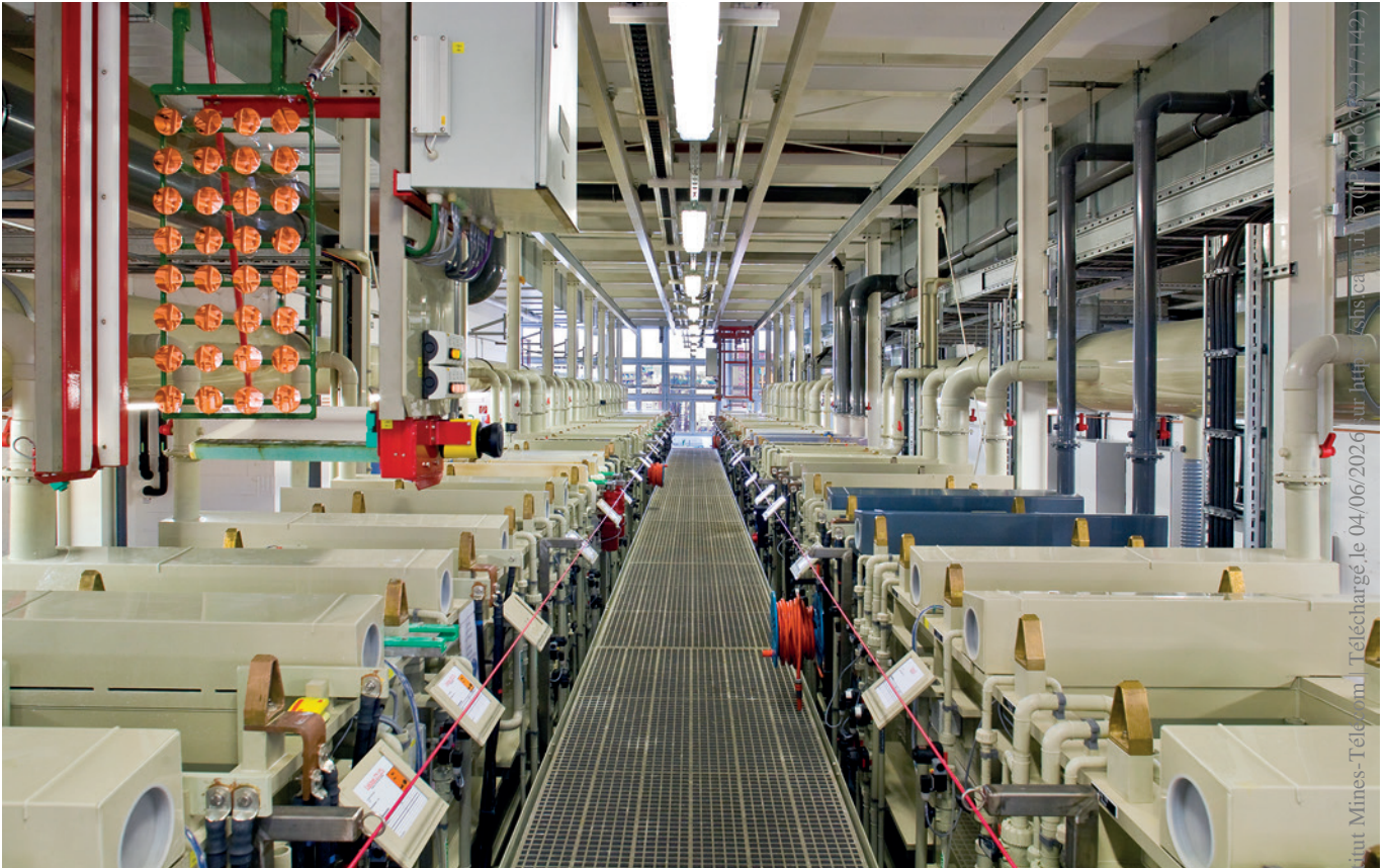
General Metal Finishing: Plating on Plastics pilot line installed in Berlin Tech Center for development, customer samplings and qualification runs for automotive industry.
